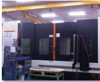
Vertical Machining Center (SVC2000)
